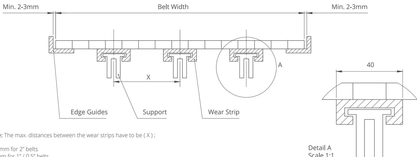
Note: The max. distances between the wear strips have to be ( X );
